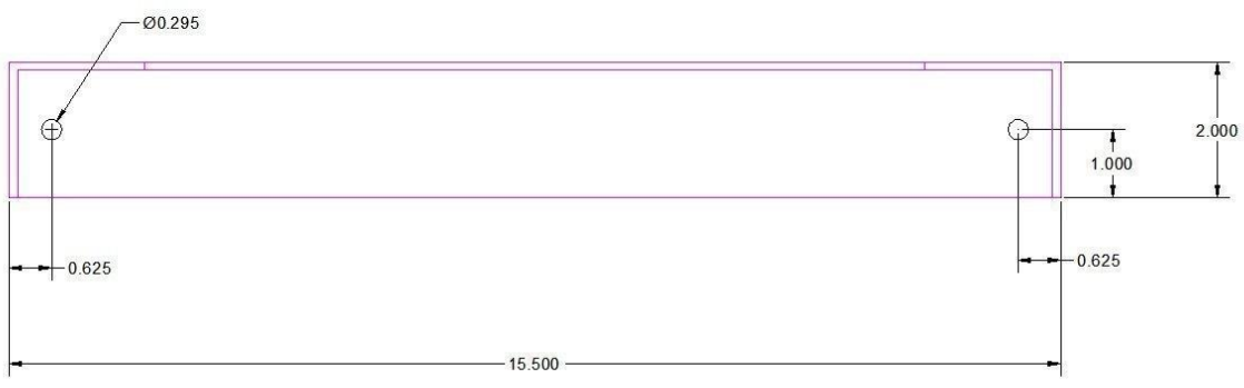
Upper Shelf with Rotor Shelf Mounting Holes (2)
